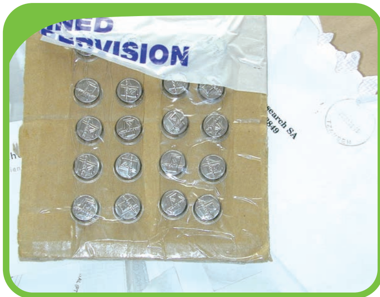
Figure 38: Electronic temperature loggers can be used to log orchard temperatures. A logger is placed in the canopy of one or two trees per orchard block. In each of a number of varieties, a set model has been determined.
